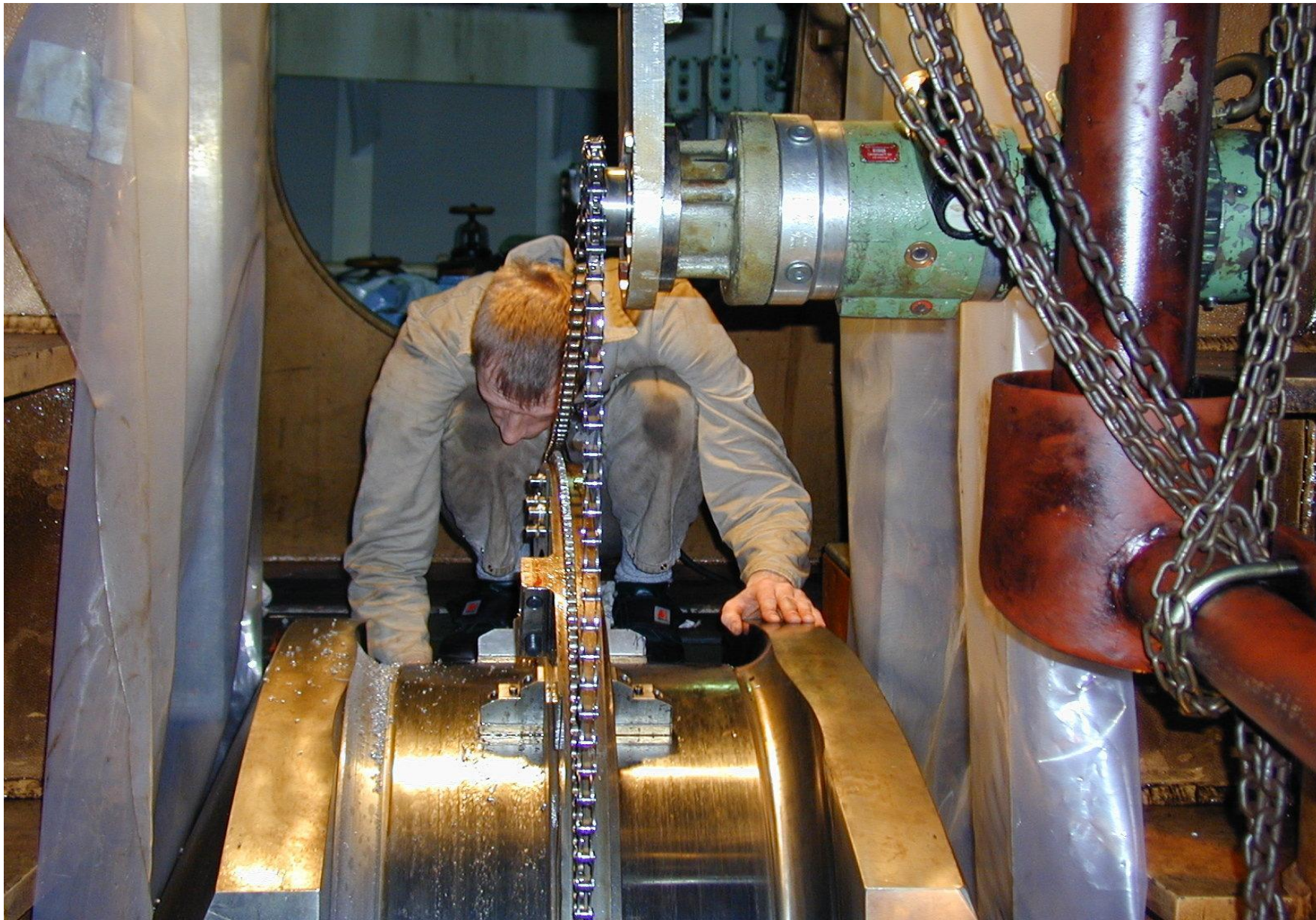
Crankpin and main bearing journal diameter machining
