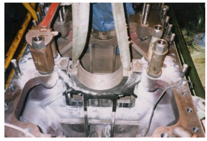
Insert being lowered into the prepared aperture making sure all the ribs are inline
