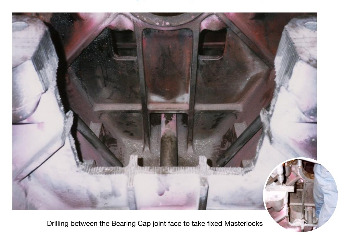
All sharp edges removed to eliminate stress raisers
